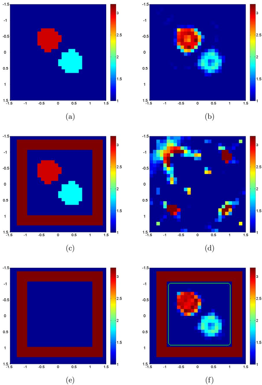
FIG. 3. Panels (a) and (c): pixel values of the relative dielectric permittivity  $\varepsilon_r$  of the phantoms shown in Figure (a) and Figure (b), respectively. Panels (b) and (d): corresponding reconstructions provided by homogeneous CSI. Panel (f): reconstruction of the phantom in (c) provided by inhomogeneous CSI, when the background is assumed to be as shown in panel (e).
