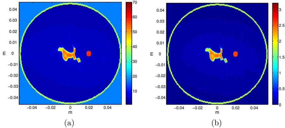
FIG. 4. Numerical phantom of the breast slice utilized in our scattering simulations, performed at a frequency of  $f = 3$  GHz. Panel (a): pixel values of the relative dielectric permittivity  $\epsilon_r$ . Panel (b): pixel values of the conductivity  $\sigma$ . In both panels, the tumoral mass is the small disk centered at  $(0.02, 0)$  m and with a diameter of 0.5 cm.
