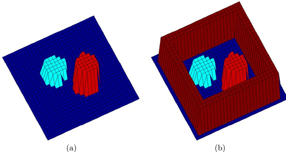
FIG. 2. Visualization of the relative dielectric permittivity  $\varepsilon_r$  of the numerical phantoms utilized for the first set of scattering experiments. The phantoms are piecewise homogeneous and purely dielectric, *i.e.*, nonabsorbing.
